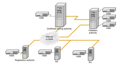
Figure 4: A multi site system protected by an nCipher Security World
